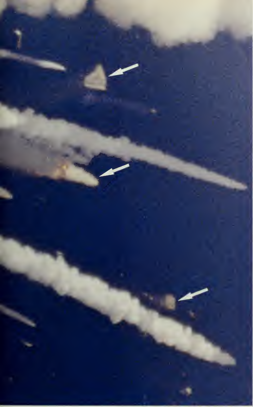
Hurling out of the fireball at 78 seconds (left) are the Orbiter's left wing (top arrow), the main engines (center arrow) and the forward fuselage (bottom arrow). In the photo below, it plunges Earthward, trailed by smoking fragments of Challenger.
